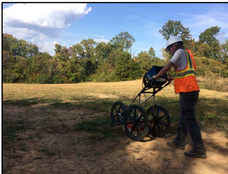
Figure 2: Jeremy Pye using the GSSI SIR-3000 GPR unit to collect geophysical data near the southeast corner of Block 1 north of Mars Hill Cemetery, view northeast toward the large brush pile northeast of the project area.
